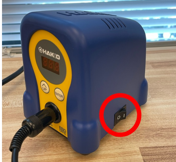
Figure 2. Picture of the soldering station control unit indicating the location of the ON/OFF switch.
